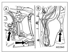
19.9 Windscreen/tailgate washer reservoir securing bolts (arrowed)
